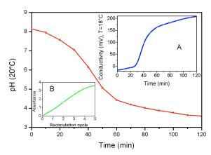
Fig. 6. pH variation on RY84 ozonation. Inset A: Conductivity variation on RY84 ozonation. Inset B: Accumulation of ozonation by-products along with RY84 ozonation-reuse cycles.
