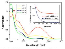
Fig. 5. UV-Vis spectra variation on RY84 ozonation processes. Inset: Decolorization and decomposition behavior of RY84 under ozonation.
